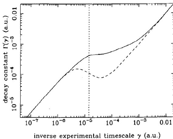
Fig. 2. Quasi-dissipative behavior in the heavy mass barrier problem (see text): (solid line) decay constant  $\Gamma(\gamma)$  versus inverse experimental time scale  $\gamma$ ; (dashed) first-order approximation  $\Gamma_1(\gamma)$ , eq. (10); the dotted line denotes  $\gamma^*$ .
